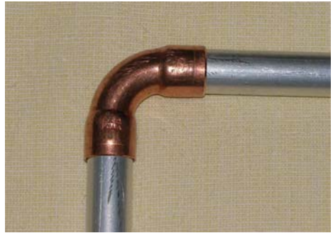
Standard copper pipe fittings from your local plumber are used.
